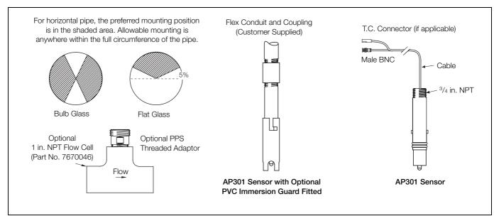
Fig. 2.2 Installing the AP301
