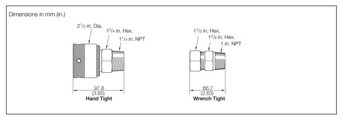
Fig. 1.4 AP304/5 Compression Fitting Dimensions
