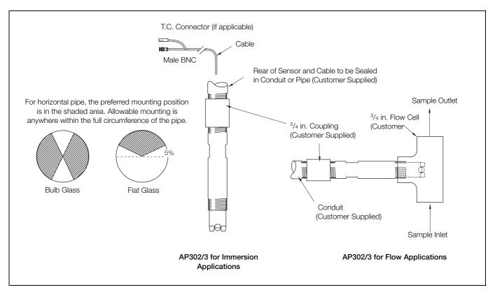
Fig. 2.3 Installing the AP302/3
