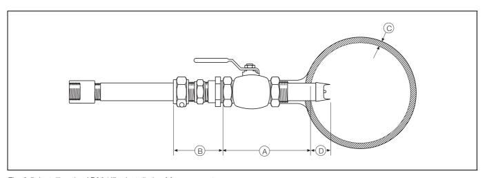
Fig. 2.5 Installing the AP304/5 – Installation Measurements
