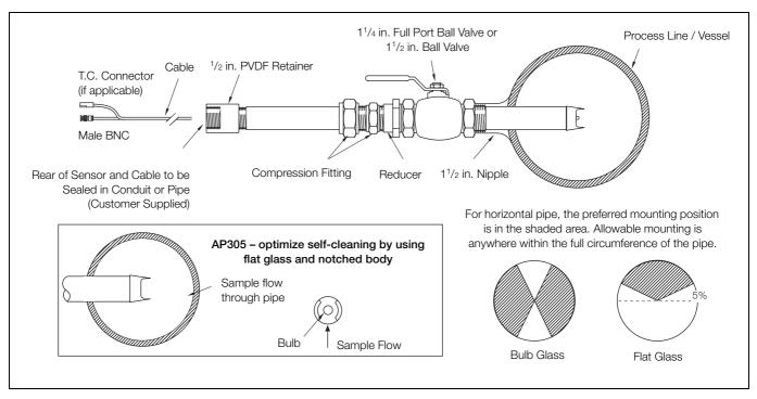
Fig. 2.4 Installing the AP304/5 - Ball Valve and Compression Fitting
