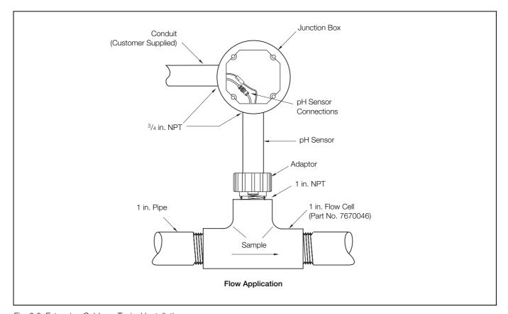
Fig. 3.3 Extension Cables – Typical Installations
