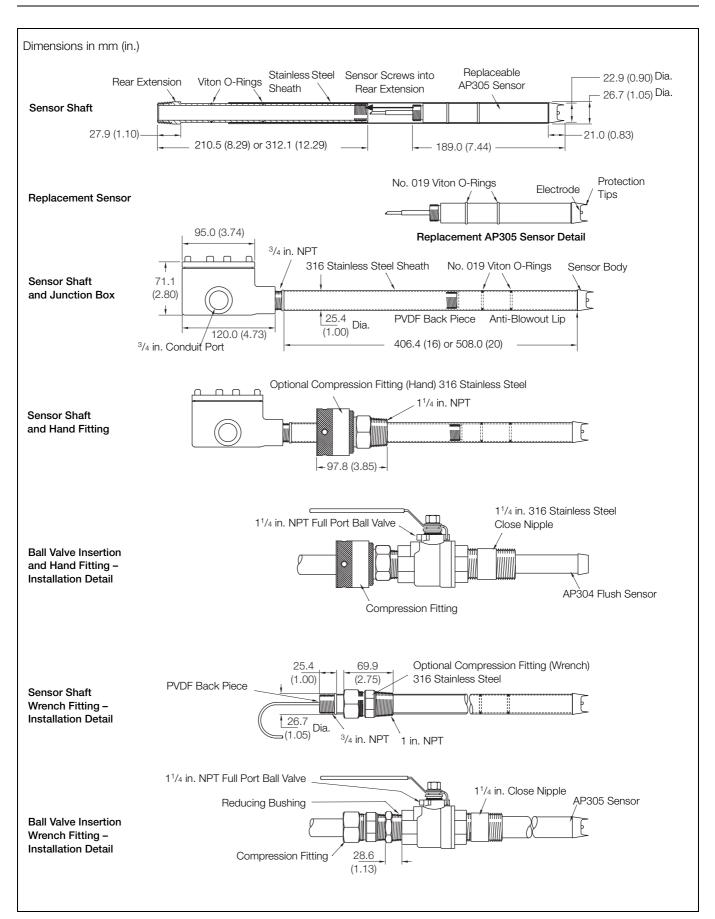
Fig. 1.5 AP304/5 Sensors and Overall Dimensions
